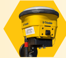
GPS/GNSS Receiver Receives data from satellites
