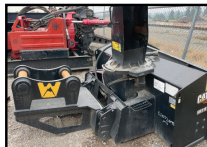
Excavator to SS Adapters
